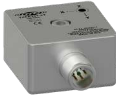
TXEA331-VT Premium, piezo velocity and temperature output, 100 mV/in/sec, 10 mV/°C, ±5%
