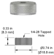
MH110-1A Ultra low profile, pull strength: 21 lbs (10 kg)
