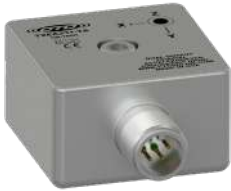
TXEA331-TA Premium, acceleration and temperature output, 100 mV/g, 10 mV/°C, ±5%
