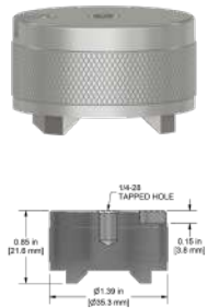
MH114-3T With triaxial locating notch, Pull strength: 50 lbs (23 kg)
