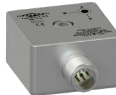
TXFA331-TA Premium, acceleration and temperature output, 500 mV/g, 10 mV/°C, ±5%
